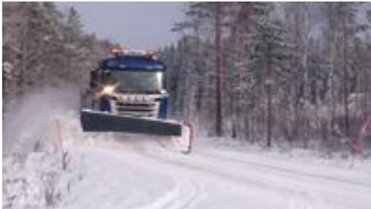
Ämteruds Åkeri's new truck is a Scania G490 8x4, featuring an Allison 4000 Series™ fully automatic transmission and two steering axles.
